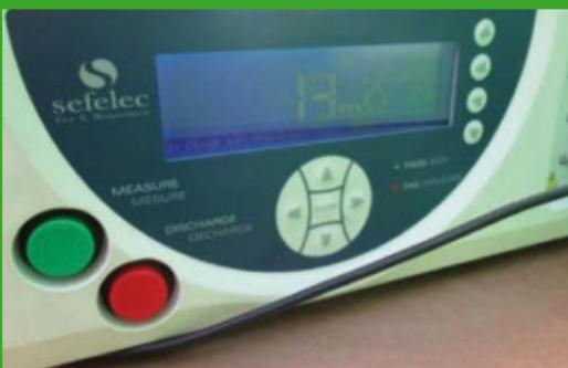
Reading of the resistance between the generator set's main protection terminal and the right-hand canopy
