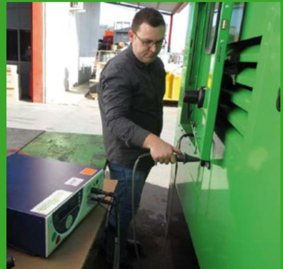
Taking measurements between the different metal parts on the generator set canopy and the main protection terminal.
