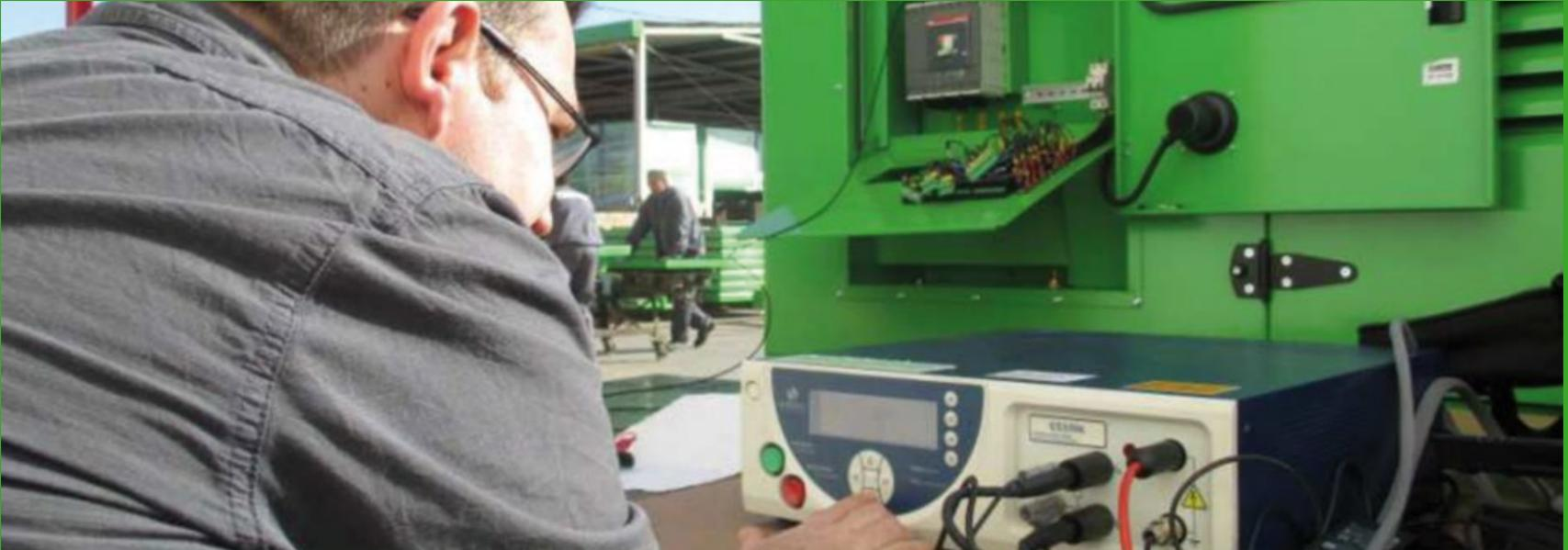
A 500 V direct current is applied using a digital multimeter.
