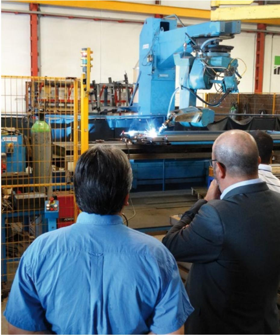
Sheet stage in Production line: Welding Robot.
